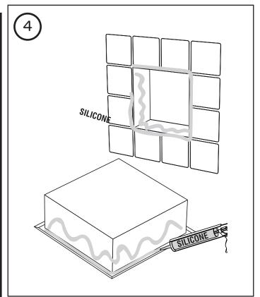
Generously apply silicone on all sides, on the inner surface of the edge of the niche, on the wall, and on the uprights (as illustrated) for optimal sealing support.
