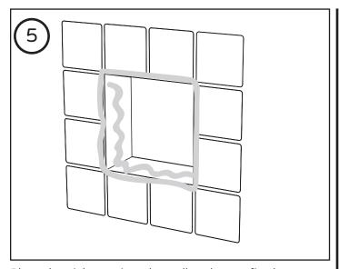
Place the niche against the wall and press firmly. Remove the niche and add silicone if it does protrude slightly.
