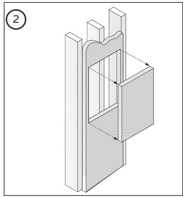
Prepare an opening between the uprights according to the dimensions X and Y of your niche, minus 1/4" (6mm). Ideally, when you insert your niche, it should offer a little resistance in the drywall to prevent it from moving until the silicone dries completely. If you have added another ceramic style finish, make it finish slightly shorter than the drywall.
