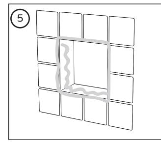
Place the niche against the wall and press firmly. Remove the niche and add silicone if it does protrude slightly.
