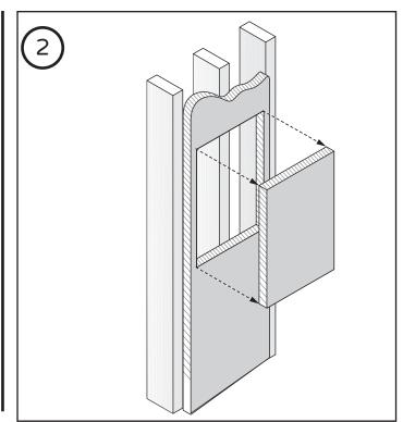
Prepare an opening between the uprights according to the dimensions X and Y of your niche, minus 1/4" (6mm). Ideally, when you insert your niche, it should offer a little resistance in the drywall to prevent it from moving until the silicone dries completely. If you have added another ceramic style finish, make it finish slightly shorter than the drywall.
