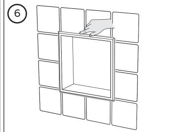
With a wet finger, wipe off any excess silicone.
