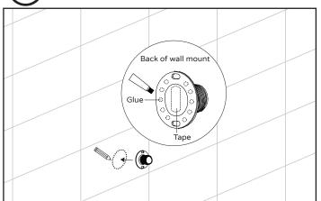
Apply glue to wall mount as indicated and add tape (included) to secure to wall. Let glue cure for 48 hours for complete result.
