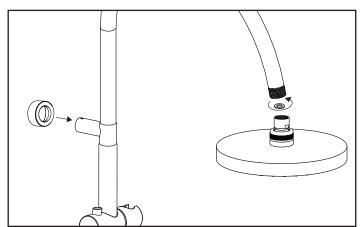
Slide escutcheon (5), insert washer (11), and screw showerhead (1) to shower arm (2) and secure.
