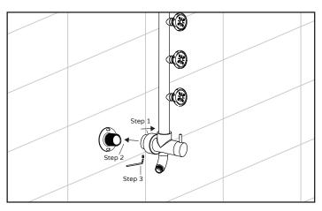
Step 1: Slide escutcheon (5) back in order to place set screw (4) later on.
