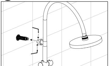
Attach assembled shower to inlet nipple and secure set screws (4) with allen wrench (18) provided.
