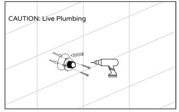
Drill wall mount (15), place it on marked location and mark holes for drilling. Set wall anchors (17) in place. Place the wall mount (15) on marked location for easy, steady, installation. Drill mounting screws (16) into place.
