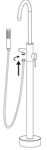
6. Install the hose to the hand shower and the tub filler. Please check the tub filler spout and hand shower water flow and its function.
