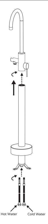
3. The flexible hoses through the straight tube. Twist tight to attach flexible hoses to faucet.
