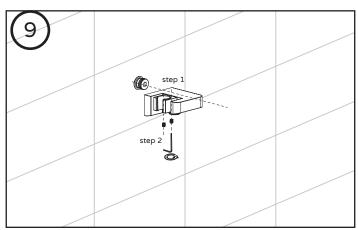
[Step 1] Push the handshower holder into the nipple. [Step 2] Use the allen wrench to tighten the setscrews at the bottom of the handshower holder.
