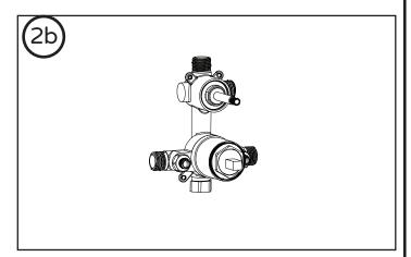
If no tub, keep the tub spout cap. Apply plumbers tape on all joint threads needed.
