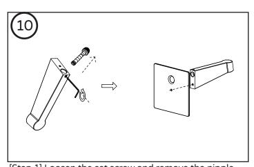
[Step 1] Loosen the set screw and remove the nipple from a shower arm
