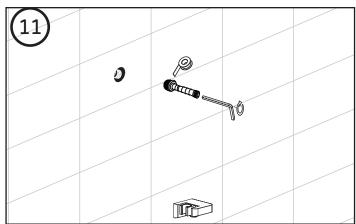
[Step 1] Place plumbers tape on nipple threads. [Step 2] Screw in nipple into plumbing and thread.
