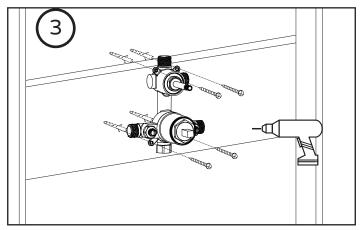
Drill screws to stud to fix main valve body.
