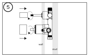
Install diverter trim sleeve and valve trim sleeve. Screw in trim nut.
