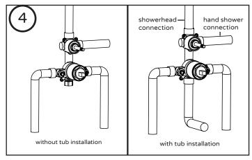
Connect the supply line to the valve, turn main water valve on and confirm there is no water leakage.
