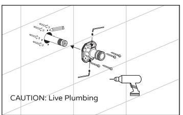
Remove set screws (2x) from Top T (15) and remove inlet fitting.
