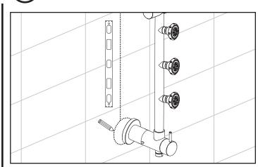
Use level to assure shower pipe is straight and mark lower diverter (24) mount location.
