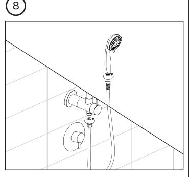
Insert washer (17) into the hex end of the hand shower hose (22). Attach hose to handshower outlet located on the bottom of the diverter (24).
