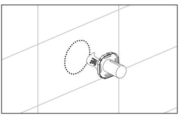
Hold for about 30 seconds to dry. Tape will be fully cured after 24 hours.
