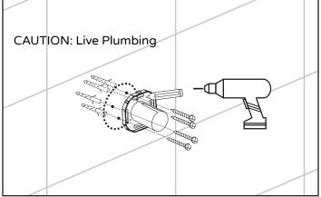
Place lower mount plate (27) on marked location and mark holes for drill option.
