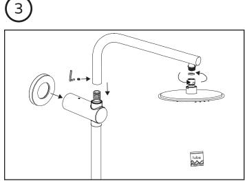
Remove plastic cover and slide shower arm (16) onto Top T (15). Connect showerhead (18). Slide in escutcheon (11). Screw showerhead (18) onto shower arm (15).
