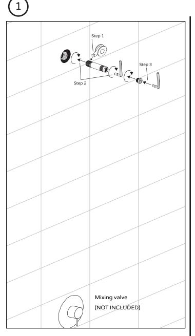
[Step 1] Apply a generous amount of PTFE (plumber's) (2) tape to end of end of nipple (4).
