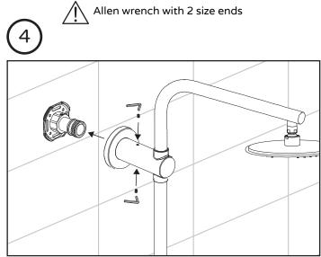
Slide in Top T (15) and secure with set screws (14).
