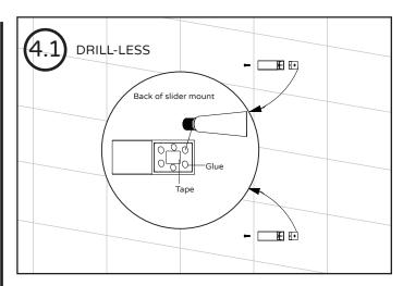
Decide where the slide bar mounts will be placed. Remove the tape cover and apply a good amount of glue on the mounting hardware. Place the slide bar mounts on the marked area, hold in place for a few minutes and let the glue cure for about 48 hours. DO NOT place the slide bar or handshower until glue is fully cured.
