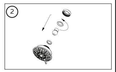
Assemble showerehad swivel joint. Once assembled connect to the showerhead.
