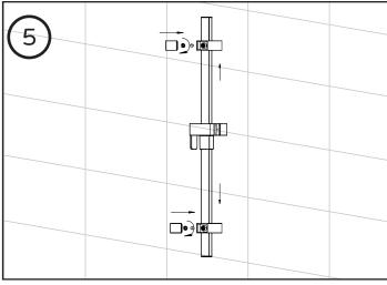
Place slide bar onto mounts. Screw into place and install cover plates.
