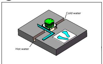
Confirm position for the mounting base (10) and standing place. Suggested distance between them is 30". Dig hole based on the mounting base (10) size.
