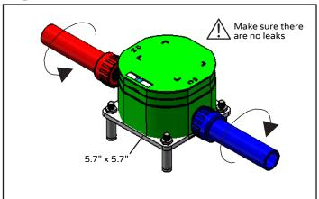
Connect hot and cold water pipes to mouting base (10).
