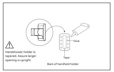
Apply glue to the handshower holder (14) as indicated and add tape (included) to secure onto wall. Let it cure for 48 hours for complete result. Handshower holder is tapered. Assure larger opening is upright.
