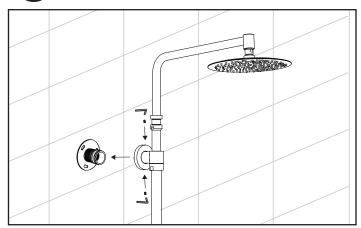
Secure shower bar to fitting and secure with set screws.
