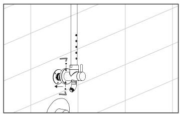
Slide bottom diverter (16) onto diverter mount (8) and secure with set screws.
