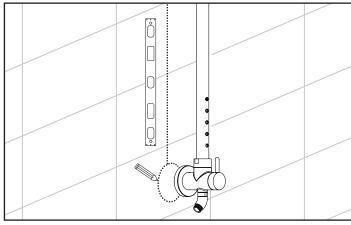
Use level to assure shower pipe is straight and mark lower diverter mount location.
