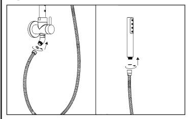
Insert washer (2) into the hex end of the hand shower hose (15). Attach hose to hand shower (13) outlet located on the bottom of the diverter (16). Insert washer (2) into the tapered end of the hand shower hose (15) and attach the hand shower (13). Place the tapered end of the hose into the hand shower holder (14).
