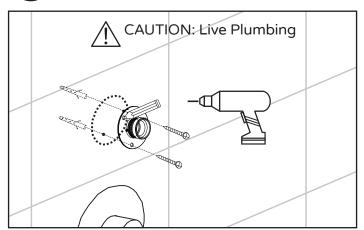
Place lower mount plate (8) on marked location and mark holes. (1 screw should be on the left side and one on the right side)
