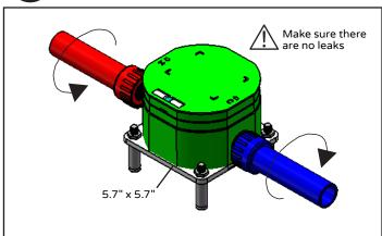
Connect hot and cold water pipes to mouting base (10).
