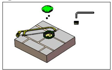
Discard mounting base cover and plugs for hot and cold water outlets. Cut the extra top part of the mounting base (10).
