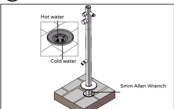
Insert bottom shower pipe (2) to the mounting base (10). Connect bottom flange to mounting base (10) with the four 5mm screws (6), then push down the bottom escutcheon.
