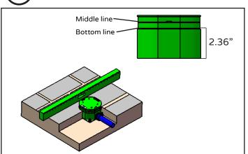
Make sure the mounting base (10) is vertical and centered to you. Tighten mounting base (10) with metal screws (11), make sure floor tile must be higher than bottom line and lower than middle line of mounting base (10).
