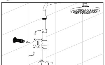
Attach assembled shower to inlet fitting (6) and secure set screw (4) with allen wrench (18) provided.
