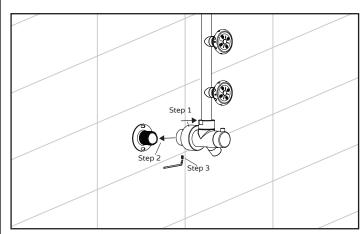
Step 1: Slide escutcheon (5) back in order to place set screw (4) later on.
