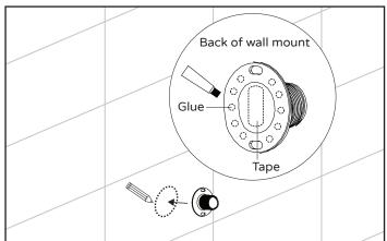
Apply glue to wall mount (15) as indicated and add tape (included) to secure to wall. Let glue cure for 48 hours for complete result.
