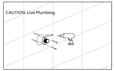
OPTIONAL: If you wish to drill wall mount (15), place it on marked location and mark holes for drilling. Set wall anchors (17) in place. You can follow Step 6 to place the wall mount (15) for easy, steady, installation. Drill mounting screws (16) into place.
