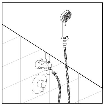
Insert washer (11) into the hex end of the handshower hose (12). Attach hose (12) to handshower outlet located on the bottom right of the diverter body (13). Insert washer (11) into the tapered end of the handshower hose (12) and attach the handshower (10). Place the tapered end of the hose into the hand shower holder (9).
