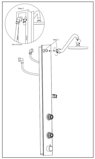
[Step 1] Secure shower arm (2) onto unit by tightening brass nut (6) on the back of unit.
