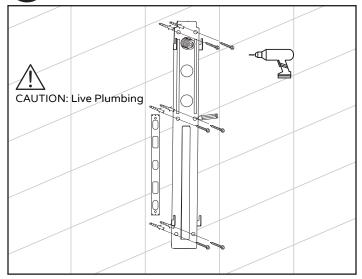
Place mounting plate (12) onto nipple (13), depending on your desired height. Use plate as a guide, mark and drill the holes deep. Insert anchors (15) into holes and secure mounting plate (12) with screws (16). Level plate before drilling. NOTE: anchors provided are for solid surface walls; If you have fiberglass walls with no backing, toggle anchors must be used (not included).
