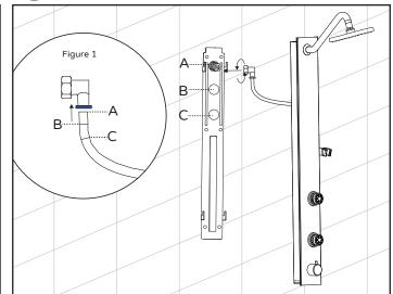
Connect main supply line (9) to brass nipple (13).
