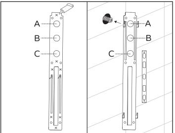
[Step 1] Remove face of tape (14) from mounting plate (12), apply glue (25) as shown and slide plate over nipple (13) through predetermined hole (A,B,C).
